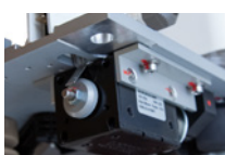
ELECTROMAGNET LOCK SYSTEM
